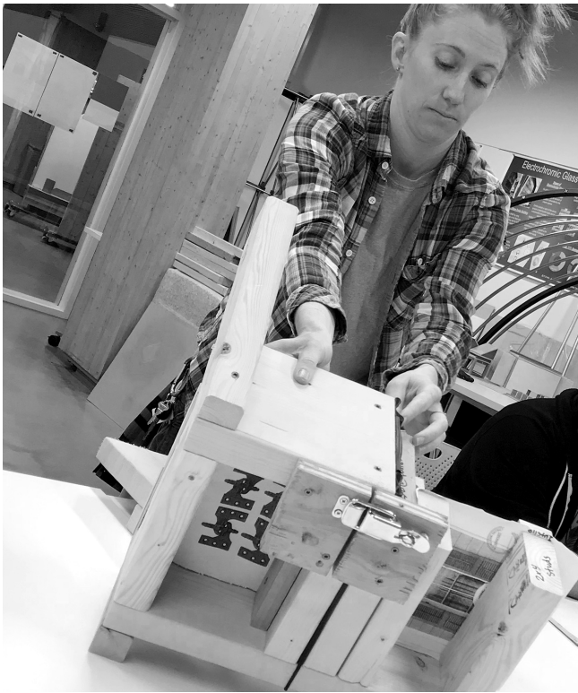
Figure 4. Testing panelized construction joints. Photograph by author.
